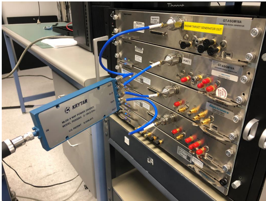
Photo 1 showing the four channels of ASGs summed using a power combiner
