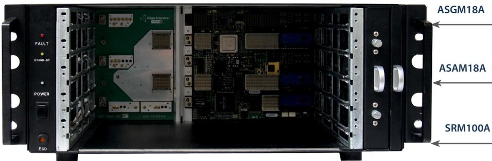
CHSIS2A AXle System Chassis (4U) (For 1 to 2 channel systems)
